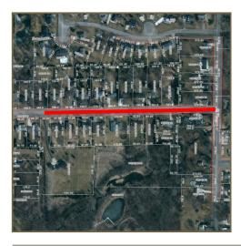
**Description & Scope:** Sheldon Road is in need of ditching and culvert work along the north and south ditches. Scope of work is anticipated to include new stormsewer, inlets and culvert/apron replacement.
