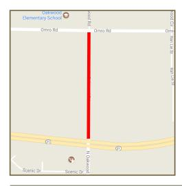
**Description & Scope:** Last resurfaced in 1995, N. Oakwood Road has completed its regular surface longevity and is due for work greater than crack and road sealing. A 0.31 mile stretch from STH-21 to Omro Road is proposed. Existing road surface is 22' wide and within a 66' right-of-way. Proposed improvements include manhole adjustments, binder mat and wedging, limited patching, asphalt replacement and striping.
